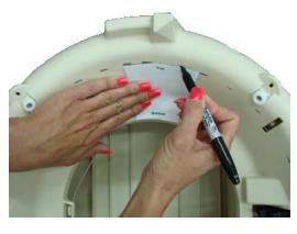
Base Seal Installation for base without Rib: Cut out the template on the reverse side of this sheet and place it on the base as shown (left). Make frequent marks the protective strip and place the base strip above the line you have created (right). Lastly, press down firmly on the seal strip.
