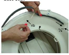
Base Seal Installation for base with Rib: Peel back the protective strip and place the base seal strip above the rib (left). Then, press down firmly on the base strip. The base seal strip should look like the picture to the right when installation is complete.
